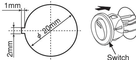
※ If the hole is bigger than 20mm diameter, the switch does not fix stably. Recommend to make a smaller hole, then adjust the size by inches.
