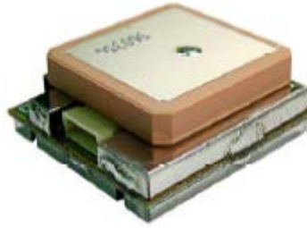
Figure 15. EM406-A GPS receiver module [11].
