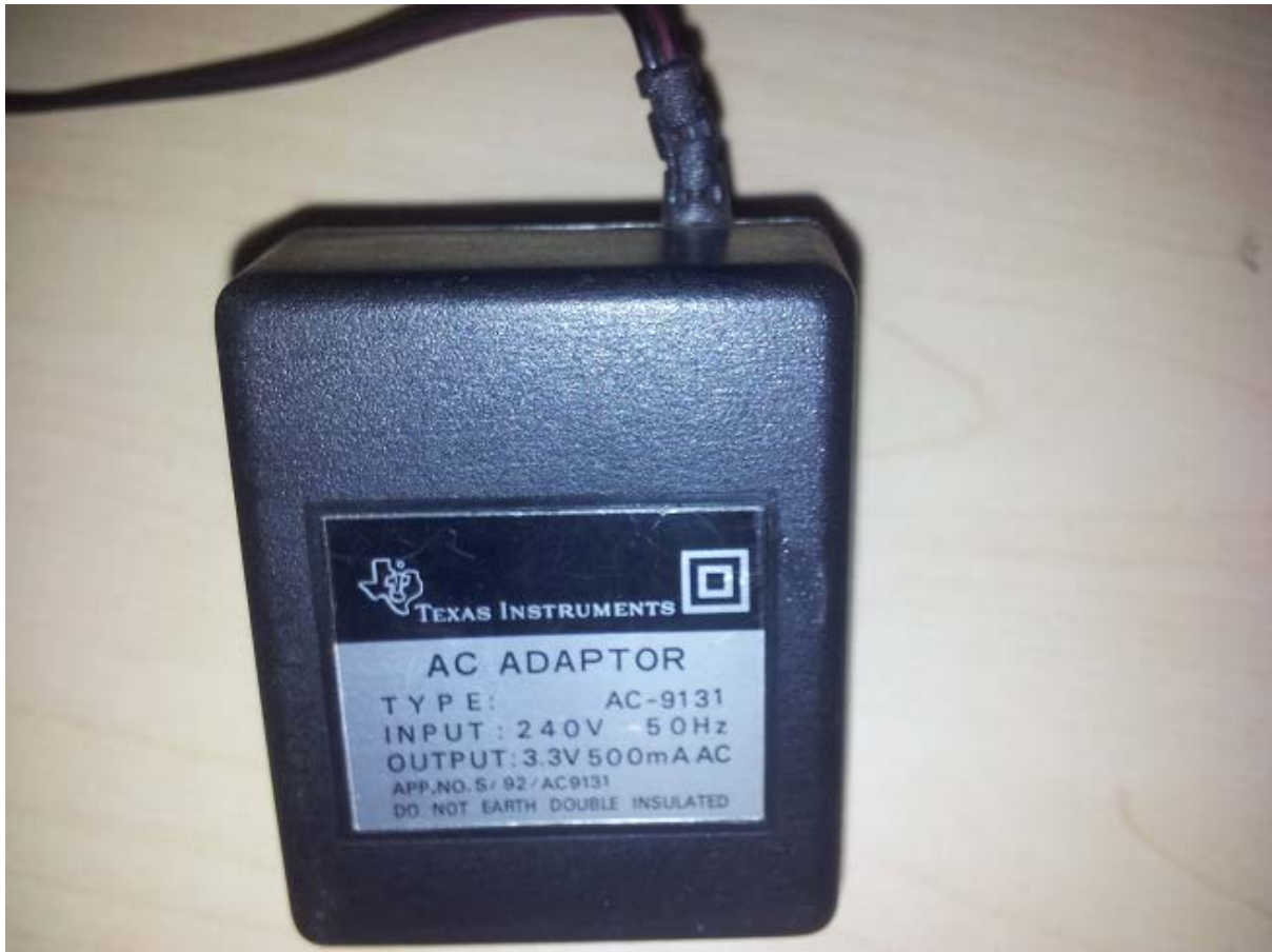
Figure 9. TI AC-9131 AC-AC step-down conversion adapter.
