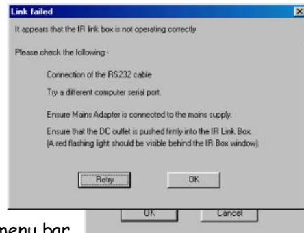
To change the prescribed serial port, click on **OK**, select **Hydrosteel**, and from the 'ISL Instrument Interface window menu bar, select **Settings, Port**. Click on an alternative serial port (usually Com 1 or Com 2), click **ok**, and close the 'ISL instrument interface menu panel. Return to step 4.
