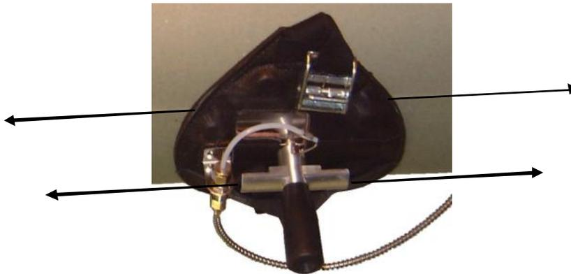
indicator runs in the same direction as the pipe or axis of the vessel, as illustrated. Confirm the probe's flexible plate conforms snugly to the steel surface. On piping of less than 8 inches diameter, use the strap provided. The strap should be drawn tight as shown below, so as to ensure the probe plate is tight against the steel, when the hands are released.
