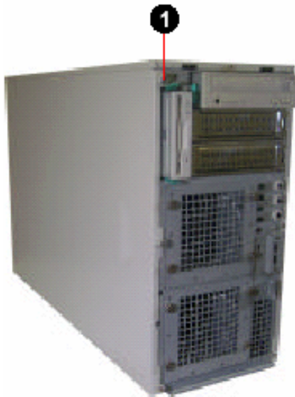
Figure 5: Removing the three thumb screws.
