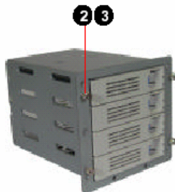
Figure 13: Installing HDD and HDD Cage
