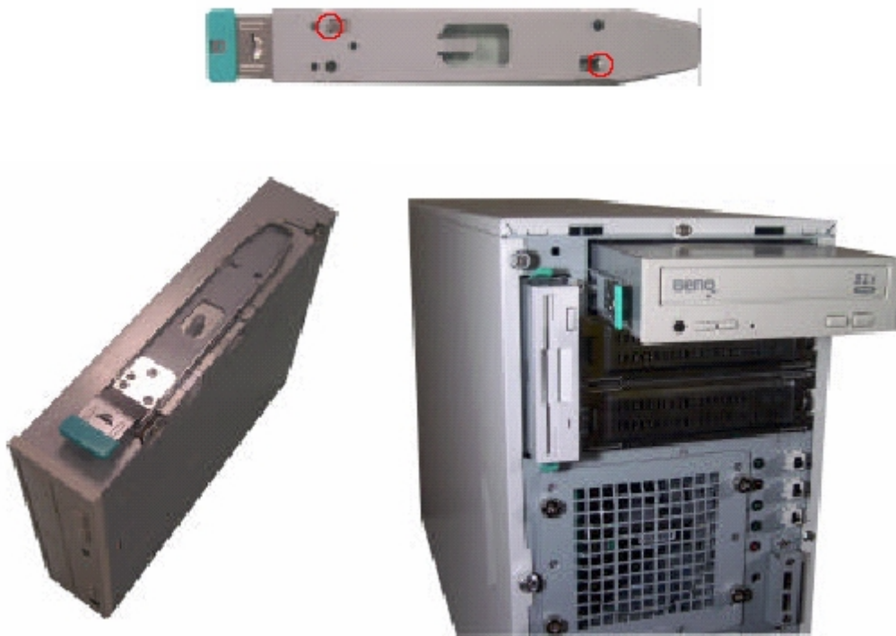
Figure 18: Installing the CD-ROM Drive
