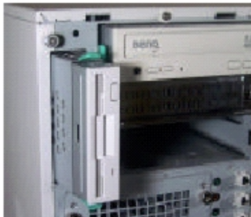
Figure 17: Installing the Floppy Drive Carrier into the Chassis
