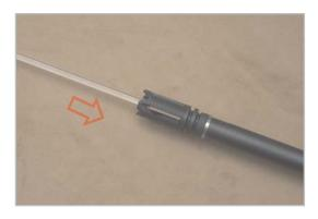
Remove the inner barrel by sliding it through the upper receiver, towards the rear of the gun.
