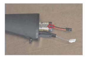
Now connect the battery by lining up the two connectors and push them together. The plugs are polarized so they will only fit together in one direction. Also make sure the lock is fully engaged.
