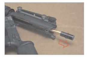
Occasionally lubricate the rubber seal and hop-up unit from the loading port of the inner barrel. Use only pure (100%) silicon oil, as many other lubricants (such as mineral oil, automotive lubricants, or WD-40) can immediately destroy the o-rings and other rubber components found within the inner
