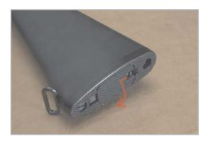
Locate the battery connector, and extract the wire until the black, tubular fuse holder is completely outside of the battery compartment. Be careful not to damage the wires. If you need to replace the fuse, use a needle nose plier to pull it out of its holder. Only replace with identically rated fuse units.
