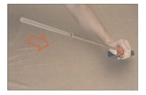
While keeping a firm grip on the magazine and loading tool, insert the provided acrylic rod into the feeding tube with your other hand. Use the acrylic rod to push the BBs through the loading tube into the magazine. You should not need to apply excessive
