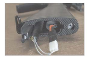
Place the battery connector and the remaining wires into the battery compartment. Close the compartment door and ensure it locks in place. Now your Systema Training Weapon is ready for use.
