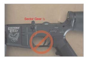
gears, tap the trigger lightly until all of the sector gear's teeth rotates inside the lower receiver (disappear from view), before you attempt to close the upper receiver.
