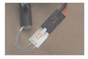
Insert the fuse holder into the available opening under the battery. Be careful not to force the fuse holder into the compartment, as you may damage the wires.
