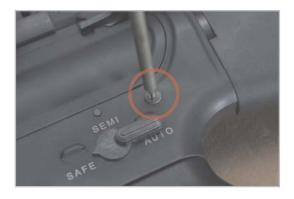
With your palm rested firmly on top of the stock, push the charging handle with your thumb to pivot the upper receiver. There is a spring-loaded ball bearing that holds the upper receiver securely in place, so a considerable force may be required to open the upper receiver.
