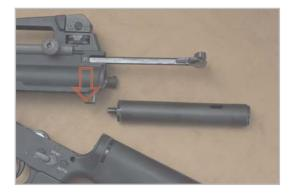
After removing the cylinder unit, the charging handle can also be removed by sliding it all the way back then moving it downwards. Replacement and upgrade cylinder units will be available from your Systema dealer shortly.
