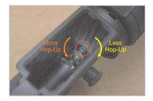
After the adjustments has been made, install the magazine and test-fire the weapon in a shooting range. Notice the trajectory and re-adjust if necessary. Please also note that every
