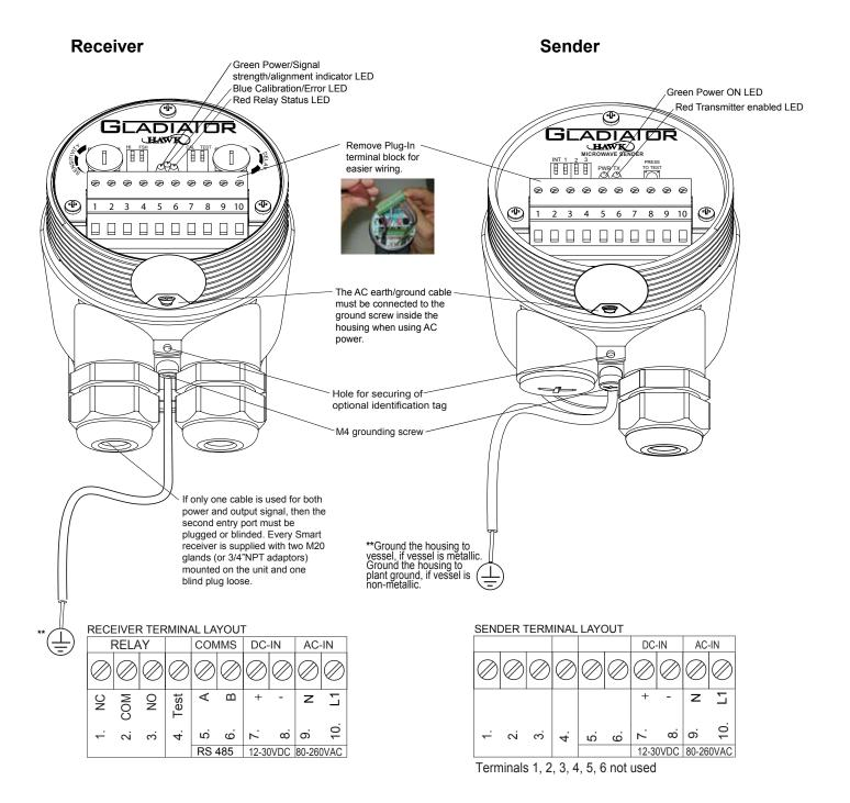
Note: AC power terminals may only be used when universal AC power supply option has been selected - see part numbers - AC terminals have no function in products without universial AC power option.
