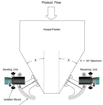
Adjustable microwave mounting bracket MA-12 or MA-13 welded to vessel wall. UHMW (MA-12) or Teflon (MA-13) Window.
