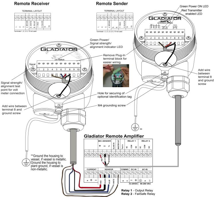
Note: AC power terminals may only be used when universal AC power supply option has been selected - see part numbers - AC terminals have no function in products without universal AC power option.
