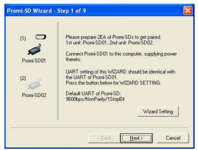
Plug SD1 into the serial port of host computer and power on. Status (Promi-SD101/202) or Standby (Promi-SD205) LED will be lit in red. It may be blinking in green if SD1 has different settings from factory defaults.
