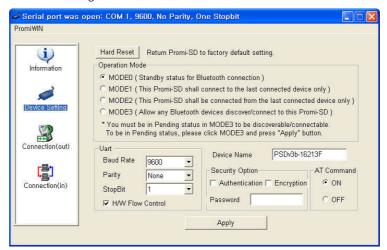
Promi-SD has 4 response messages, 'OK', 'ERROR', 'CONNECT', and 'DISCONNECT'. In some cases, these responses can affect the host system unexpectedly. To prevent this, user can set the response to ON or OFF.
