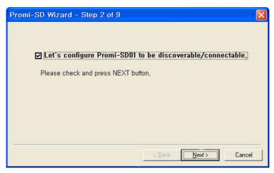
Click [Next] with marking in the check box. SD1 becomes in Scan mode, in which SD1 can be discovered and connected from other Bluetooth device. Status (Promi-SD101/202) or Standby (Promi-SD205) LED will blink twice in green every 3 seconds.
