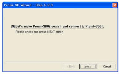
Click [Next] with marking in the check box. Status (Promi-SD101/202) or Standby (Promi-SD205) LED will blink in green. SD2 begins to search nearby Bluetooth devices for 30 seconds. The program will show the Bluetooth devices with Device Address, Device Name and CoD (Class of Device).
