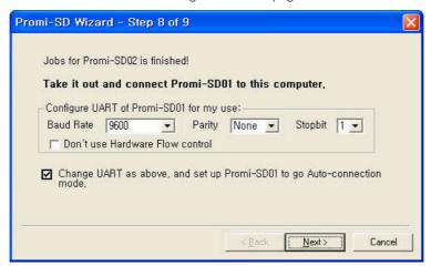
Take SD2 out of the host computer and plug SD1 into the serial port again. Set the operation mode of SD1 to Mode2. SD1 is working as a slave waiting for the connection from SD2.
