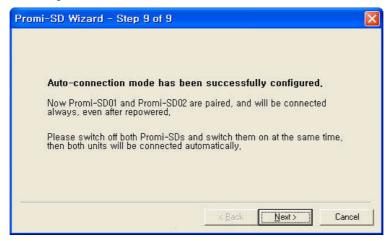
Now the configuration of SD1 and SD2 has been completed. When power off and on both of them, they will make connection again automatically.
