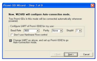
Set the operation mode of SD2 to Mode1. SD2 is working as a master trying to connect itself to SD1.
