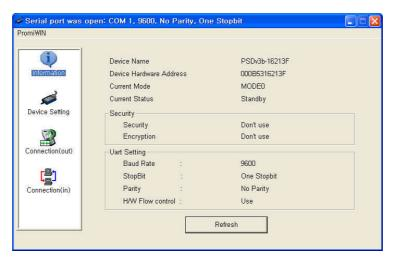
Serial port settings can be changed by <Start Configuration> and <PromiWIN Configuration> of PromiWIN in the menu bar at upper left corner of the window without re-running the PromiWIN program.
