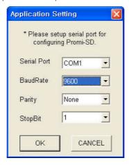
Set each option properly and click [Confirm]. If the settings are different from the host computer, error message will pop up. If the Promi-SD is in the status of connection, warning message will pop up. Then the current connection can be cancelled by [연결 해제] button on the main window.
