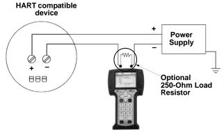
To temporarily install the optional 250 ohm load resistor:
