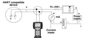
Figure 3-3 illustrates how to connect the 375 Field Communicator directly to the terminals of a HART device.
