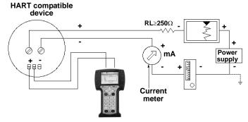
Figure 3-4 illustrates how to connect the optional 250 ohm resistor. Attaching a resistor is necessary if less than 250 ohms resistance is present in the HART loop.
