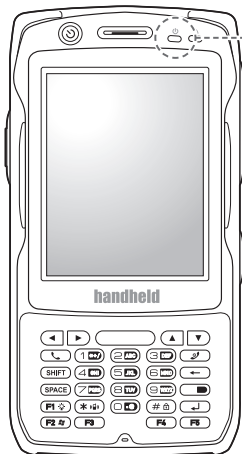
Charging indication lamp
