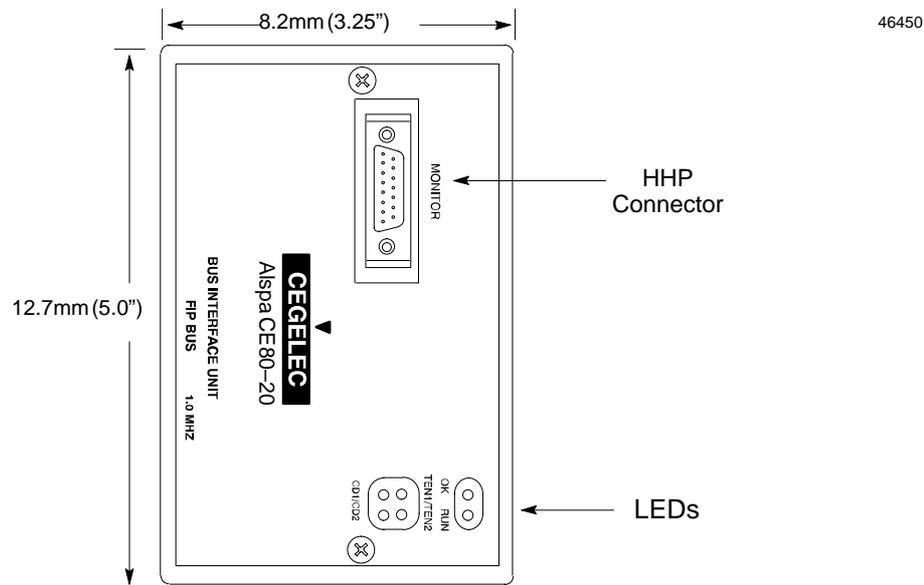
The Bus Interface Unit requires an external source of 24 VDC power.
