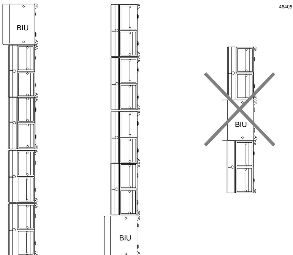
Terminal Blocks can be mounted in any orientation without derating the modules' temperature specification.
