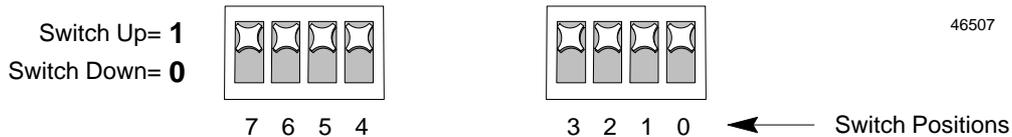
Switch 7 selects FIP or World FIP protocol, as shown in the table below. Switches 0 through 6 represent a Station ID from 0 to 127 (decimal).
