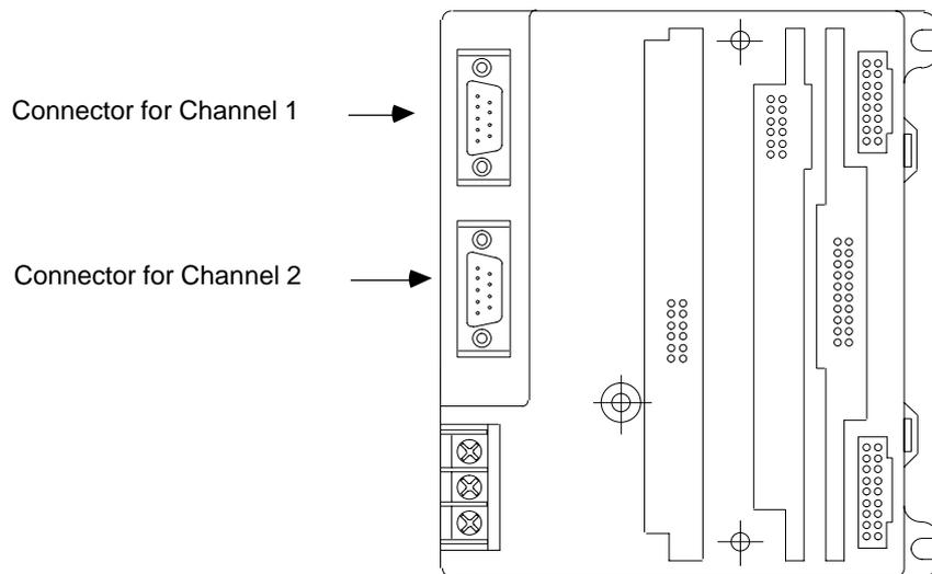
**Note:** If only one FIP bus is used, it is recommended that you cover the unused FIP bus connector with an anti-static cap.
