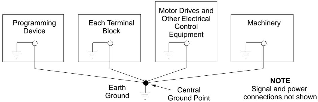
Each Alspa CE80–20 Terminal Block has a chassis ground terminal for safety and noise protection. This terminal should be connected to the conductive mounting panel with a 10 cm (4-inch) maximum length of 2.1 mm<sup>2</sup> (AWG No.14) wire. Use hardware such as star washers to ensure ground integrity.
