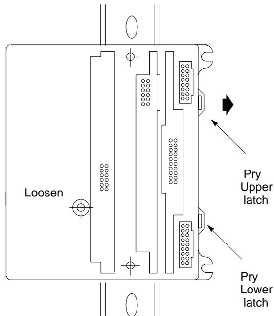
4. Keep gently pulling the top of the terminal block away from the rail. Insert the screwdriver into the lower latch and pry it outward to free the terminal block.
