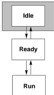
In Idle Mode, the Bus Interface Unit can indicate its presence on the FIP bus, but it cannot exchange I/O data.
