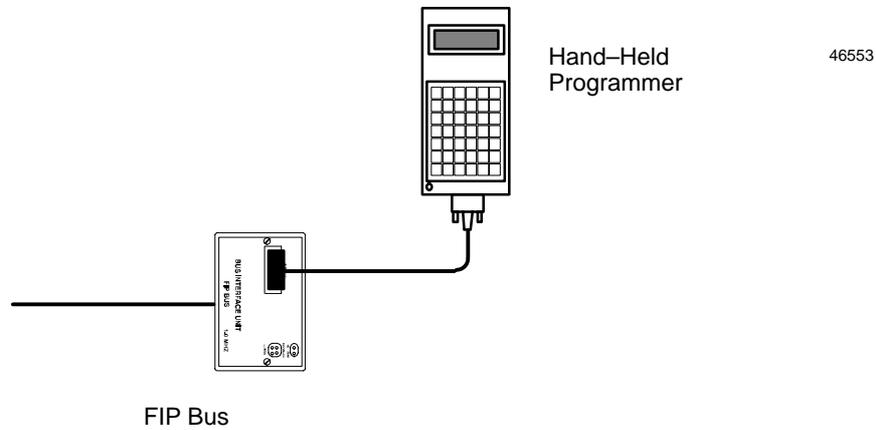
The Hand-Held Programmer can be used to monitor, force, and unforce I/O, and to display diagnostics.
