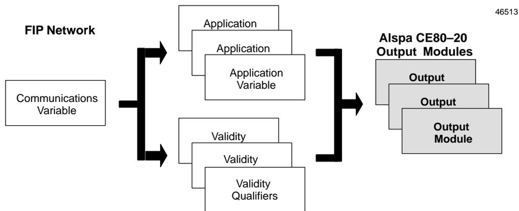
2. The Bus Interface Unit places the output data into its Analog Output table.
