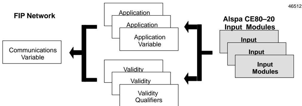
The Bus Interface Unit honors requests for input data even when the data is invalid (e.g. the corresponding input module has been removed). By monitoring the validity data, the host can know whether the data it receives from the Bus Interface Unit is real or defaulted input data.
