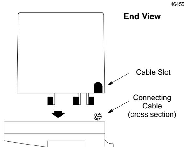
1. Before installing a new Bus Interface Unit, remove the cable slot knockout on the end of the module that will cover the connecting cable. It can be removed with pliers, or by pressing *out* from inside the module housing.
