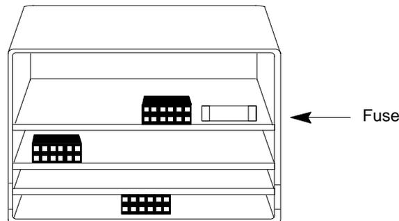
To remove the fuse from the holder, carefully pry it upward. Take care not to damage any components in the module. Place the new fuse in position and press it into the holder.
