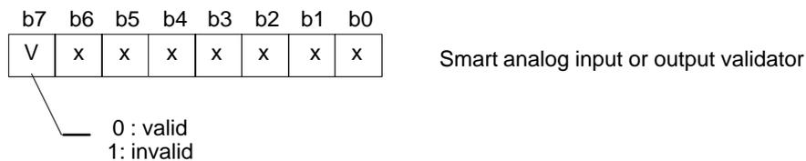
Smart I/O modules may report extra diagnostic data. The FIP BIU may be configured to decode this module's data to set up specific bits in the module's validators.
