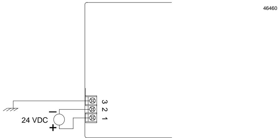
2. Connect the ground terminal to chassis ground using a 2.1 mm<sup>2</sup> (AWG No.14) stranded wire.
