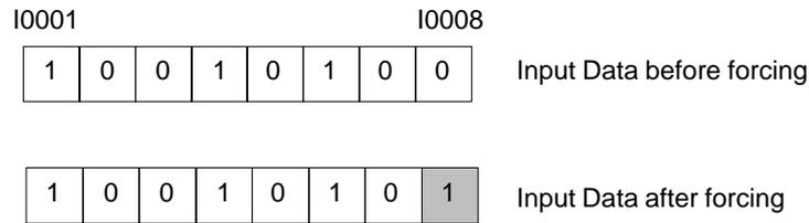
4. When you force the state of a point, the Bus Interface Unit forces the corresponding validator (IVF) to 0 (valid).
