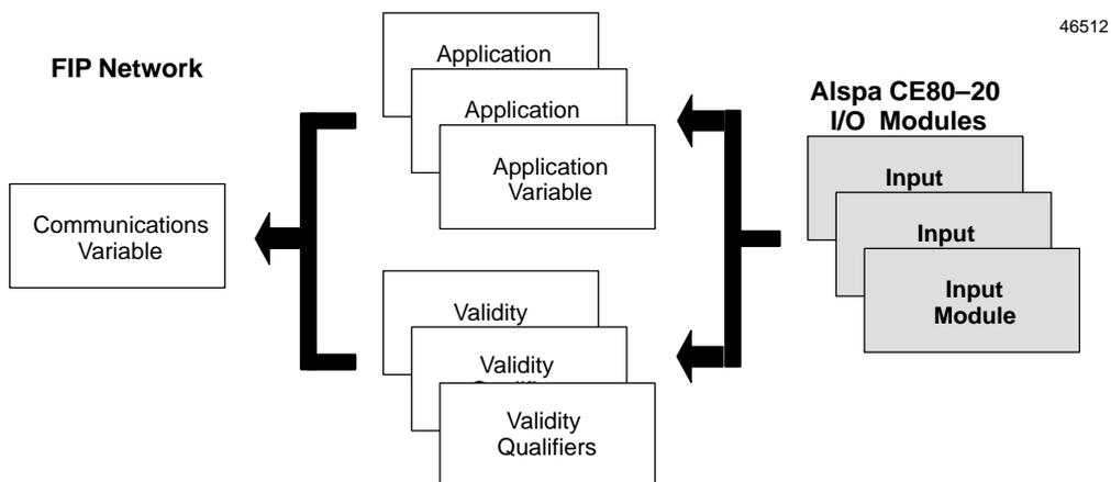
The Bus Interface Unit honors requests for input data even when the data is invalid (e.g. the corresponding input module has been removed). By monitoring the validity data, the host can know whether the data it receives from the Bus Interface Unit is real or defaulted input data.
