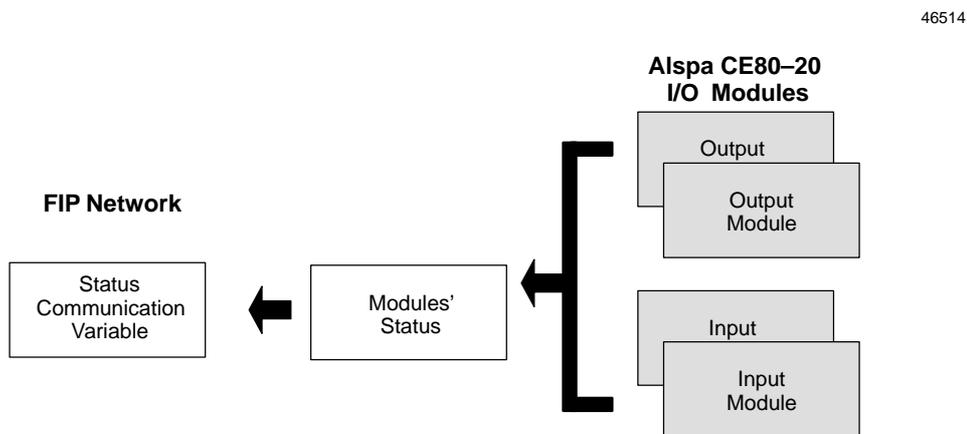
If a problem occurs (or is corrected) with any module or circuit, it is included in this status information. Such module problems do not affect the operation of the Bus Interface Unit or its communications on the network.
