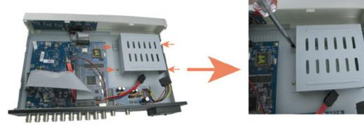
STEP 2:Remove HDD Bracket
