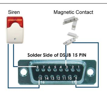
**Siren:** When the DVR is triggered by alarm or motion, the COM connects with NO and the siren with strobe starts wailing and
