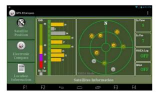
SBAS (satellite-based augmentation system) provides additional accuracy and reliability for the GPS devices. Ground stations are necessary to achieve the purpose. The SBAS feature works where such stations exist. You can enable the SBAS feature. (See "Getac Peripheral Settings" in Chapter 7.)
