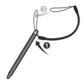
2. Insert the other loop end to the right-side holder on the device (as indicated by • below). Then, insert the stylus end through the loop (as indicated by • below) and pull it tight.
