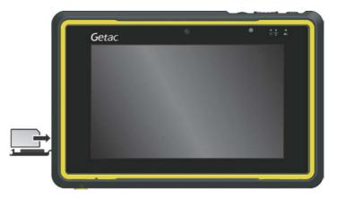
**NOTE:** To remove the SIM card, slightly push in the card to release it and then pull the card out of the slot.
