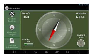
The Accuracy reading is for your reference. When the application determines that calibration is needed, it will pop up the "Calibration" graphics asking you to calibrate the compass. Hold the device and swing it in the way as shown on the screen. Do this several times until the popup graphics disappear.
