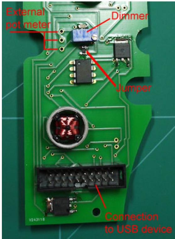
Connecting the engine device to the center USB device is very simple. Just plug in the flat cables that come with the package.
