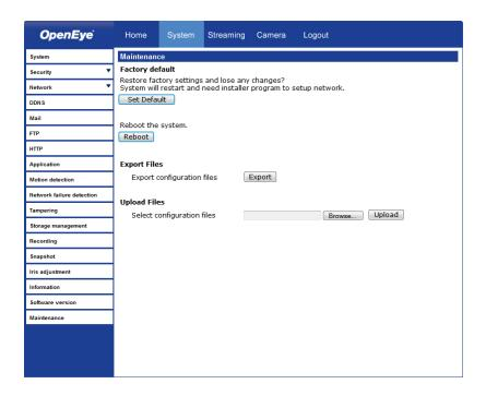
**Set Default** –To reset the IP camera to the factory default settings, including the default IP address, click Set Default. The system will restart after 30 seconds. If you cannot access the camera menu, you can return the camera to the factory default settings by holding down the reset button on the camera connection board for 30 seconds. See *Connections* for the button location.
