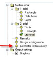
In this section, you can define the parameters required for the hot design and the rigidity calculation in the <u>accidental design situation fire</u>
