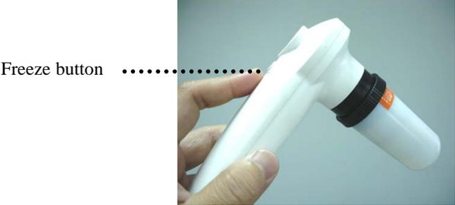
**(1) Single Frame Freeze** --- Push the mode button to Single frame freeze function
