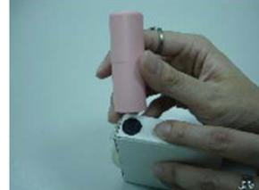
Touch properly the white plate of **moisture test bar** to the white side and the black sticker paper will be on the top of test bar.
