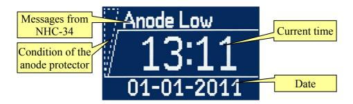
In this view the fields "Condition of the anode protector" and "Messages from NHC-34" have the same meaning. The time and date take the rest of the screen.
