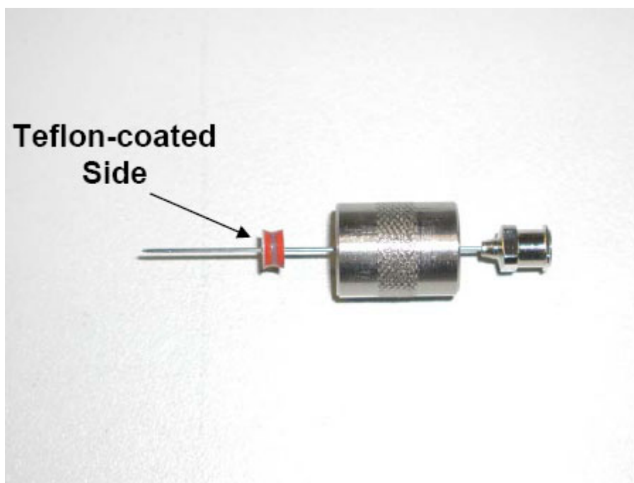
FIG. 10. Arrangement for septum predrilling.
