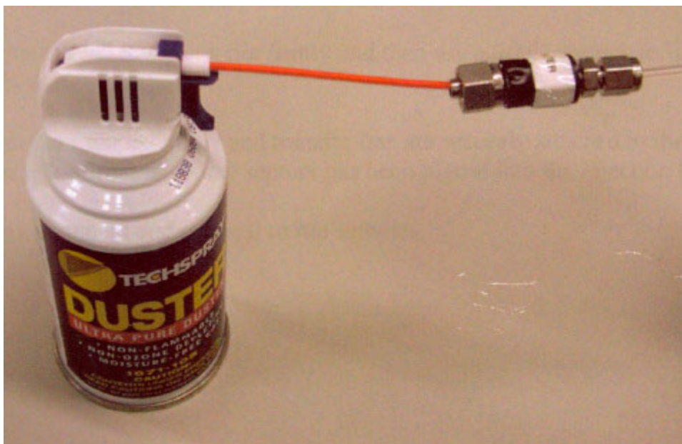
FIG. 13. Photo of compressed air set-up for cleaning the filter and line. The line is open at the septum end (not shown). Remember to blow out any septum pieces from the septum tube well area as well.
