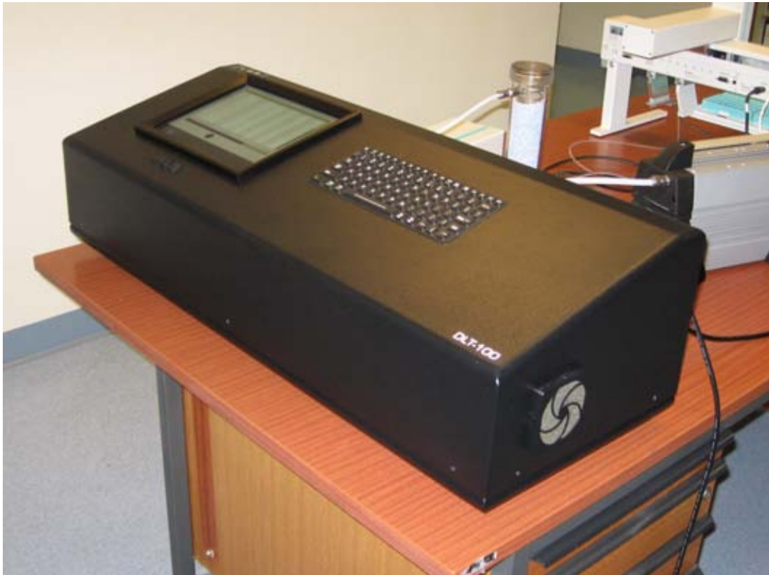
FIG. 1. The Los Gatos DLT-100 liquid-water stable isotope instrument. Vacuum pump, Drierite column and autosampler are shown in the background.
