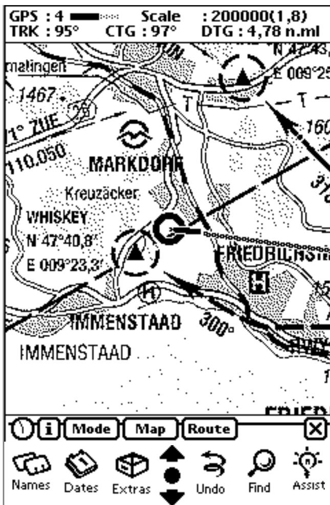
the actual position is at the center of the circle, the pointer shows to the movement direction, and the grey line is the route
