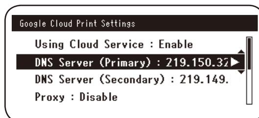
If also using a secondary DNS server, select [**Setting**]-[**Google Cloud Print**]-[**Google Cloud Print Settings**]-[**DNS Server (Secondary)**], and set the IP address.
