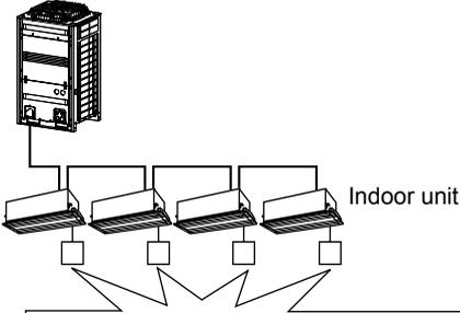
**A number of indoor units are connected to a single outdoor unit.**
