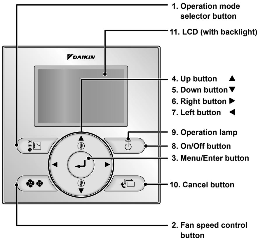
Functions other than basic operation items (i.e., On/Off, Operation mode selector, Fan speed control, and temperature settings) are set from the menu screen.
