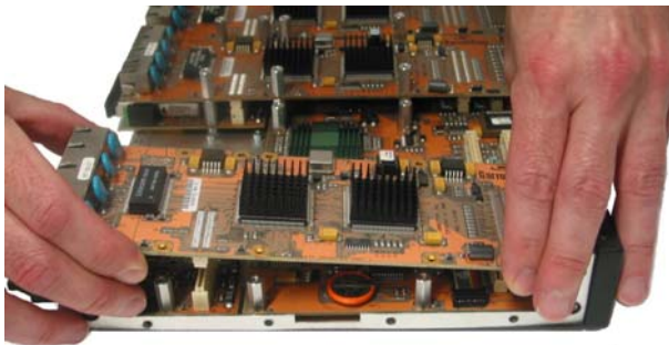
Figure 3.5.3b: Removing a 6KPM Card
