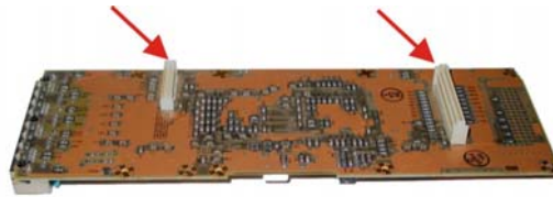
Fig 3.5.2b: Daughter Board shown upside down with two male latch connectors
