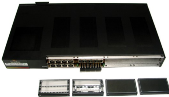
Figure 3.5.1a: Removing module panels after the screws being removed
