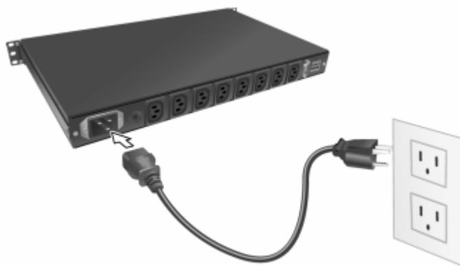
After power connected. You may see the 7-Segment LED display some error messages. If it shows “**E01**”, please refer to section 2.6 to connect IP Power Manager 8000 to your LAN or WAN. If it shows “**E16**”, that is mean the power phase of connected power outlet is reverse. Please try to make the power phase correct. Or you can refer to section 5.2.2 to disable Input Phase Detection on IP Power Manager temporarily. For other error message, please refer to Appendix A Error Code for details.
