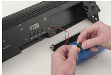
5. Carefully disconnect the battery cables.
