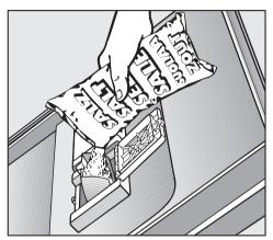
Add salt only until the reservoir is full or until water runs out of the opening. The salt reservoir holds approx. 1 kg of salt, depending on the brand used.
