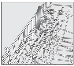
Slide the glass rack to the desired height until the catches click into place at the top.
