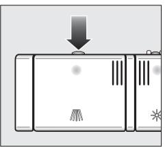
Press the opening catch on the detergent dispenser. The flap will spring open. The flap is always open at the end of a programme.
