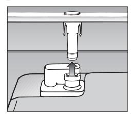
■ Pull the **lower** spray arm firmly upwards to remove it.
