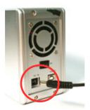
**Step 3.** Connect the square end of the USB cable to the hard drive. Then connect the flat end of the USB cable to the USB port on your computer.
