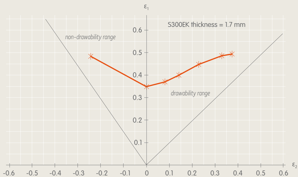
Example of FLC for a steel for enamelling
