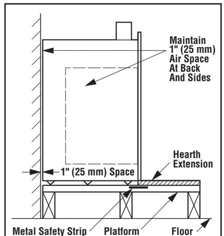
**Note:** Hearth extensions must not interfere with circulating grillwork
