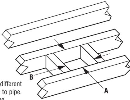
**Note:** Framing Dimensions in Canada & USA are different because installations in USA require 1" Clearance to pipe. Installations in Canada require 2" Clearance to pipe.
