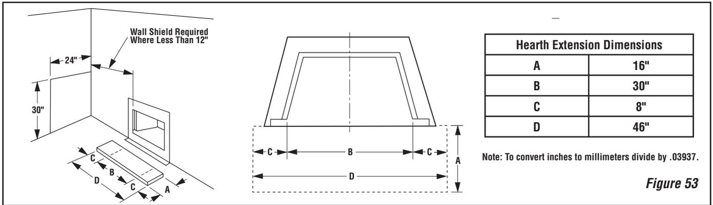
**Methods of Determining Hearth Extension and Wall Shield**
