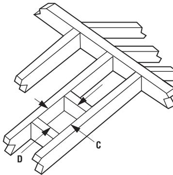
**Note:** Framing Dimensions in Canada & USA are different because installations in USA require 1" Clearance to pipe. Installations in Canada require 2" Clearance to pipe.
