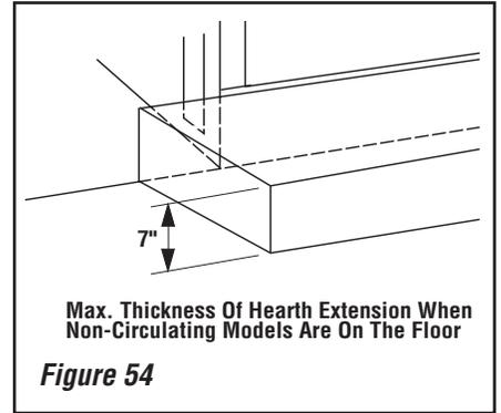
Secure the hearth extension to the floor to prevent possible shifting.
