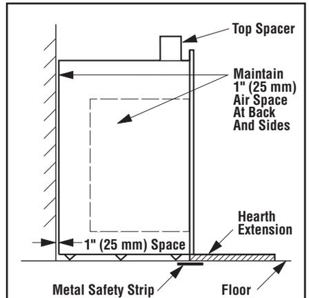
**Note:** Hearth extensions must not interfere with circulating grillwork
