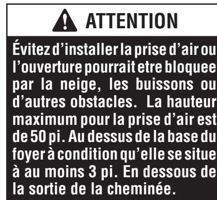
**Note:** Secure the duct hood to a vertical post with the inlet positioned downward. Ensure that nothing blocks the hood opening. This duct must never terminate higher than 3 feet below the fireplace termination (**Figure 17**).
