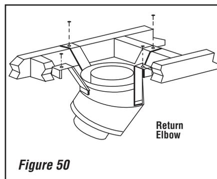
**Note:** The return elbow assembly performs the same function as a stabilizer. Consider this when determining the need for a stabilizer.
