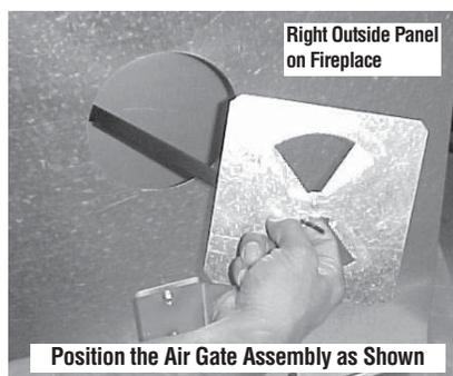
**Figure 10 - Air Gate Assembly to Fireplace**
