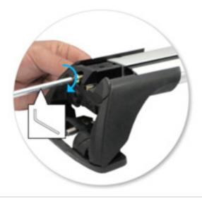
• Tighten adjusting screw to 5 Nm.
