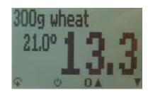
8. If the measuring value is blinking, the valid measuring range has been exceeded (limits see list on page 5). In this case the accuracy is decreasing.
