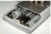
If the battery symbol appears in the measuring window resp. if a critical charge of battery is shown in the status, the batteries have to be changed IMMEDIATELY.
