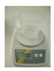
3. Switch on the moisture analyser FS3 by pressing the power button ( □ ) for 3 sec.
