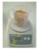
Fill up the measuring device with the sample material. The filling needs to be done slowly and constantly to ensure reproducible results.
