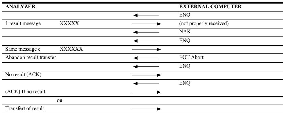
On receiving ACK, the computer need not reply. On receiving a results message, the latter must be checked (checksum) and the computer must reply ACK (06H) or NAK (15H), depending on whether the message was correct or not.
