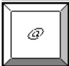
The @ key means “at” and is used for patching and setting levels on the keypad.
