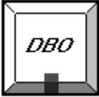
**Note that any changes caused by the Grand Master fader or DBO button are NOT reflected in the Stage Output display intentionally. If the display changed then you would have no reference as to what would happen when you restore the console to 100% output.**
