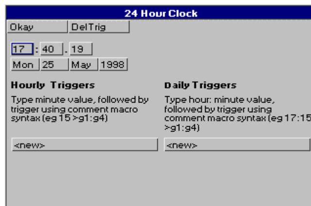
The 24 Hour Clock panel allows you to set the time and date in the console, as well as program daily and hourly triggers for comment macro style commands. The 24 hour clock and calendar in the Echelon is not affected by the Millennium bug, also known as the year 2000 bug. It will correctly change from the year 1999 to 2000, and it correctly identifies the year 2000 as a leap year.
