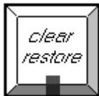
To restore the most recent contents back into the programmer, press **PIG** plus **clear restore**.
