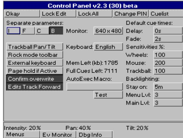
To open the Control Panel window, press **setup** followed by **Panel1**.
