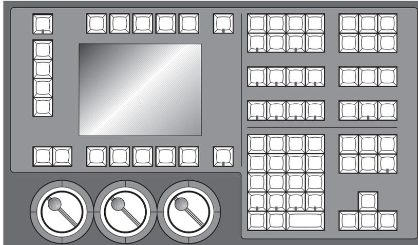
The Programmer is where cues are created and manipulated. Here, fixtures are selected, levels are set, and commands are executed. Programming is a three step process:
