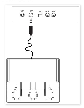
Connect the 1/4" stereo connector from the Nord Triple Pedal to the Sustain Pedal connector on the Nord Piano 2.
