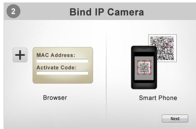
Figure 7-6 Binding IP cam to SAT Viewer
