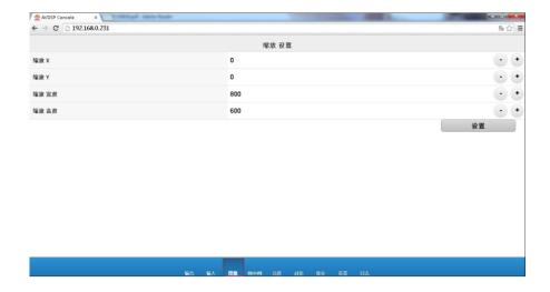
Step 5: Select "PIP" icon in title bar. When the PIP sliding block icon is grey, then it is single channel picture mode, and if image selection is gray, then image 1 is default for single image output image, and can't be chosen.
