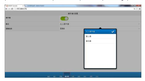
In PIP mode, the default image1 is the main image, image2 for PIP sprite, click the corresponding image when need to edit image1 or image2, the selected image with blue stripes, tick, as shown below: image2 is selected, all settings will for image 2. For example, you can switch "Input" icon in title bar to choose image 2 input source.
