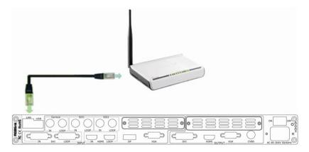
The second step: IP address setup. Please refer to IP Setup steps which in the "How to Realize LAN Remote Control Setting" section. (Make sure that processors IP address and router IP address are in the same band.)
