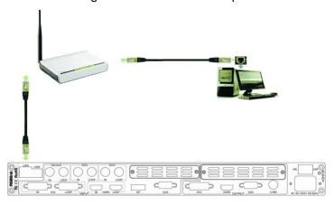
Step two: IP address setting (processor's default IP address is 192.168.0.100)
