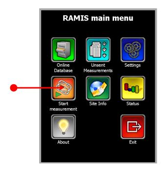
After entering the **Start Measuring** screen, first check if a heading is received. The top bar should be flashing green *and* the heading should be displayed in the middle of the screen. If this is not the case, make sure there is a Bluetooth connection to the **SPAA05** tool and that the tool has a clear view of the sky.
