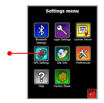
Each country uses different GPS datum and grid, so first be sure that you have selected the correct country. This will automatically set the **Datum**, **Grid and Heading** to the default settings of the operators in that country. The list with default settings can be found in **Appendix B**.
