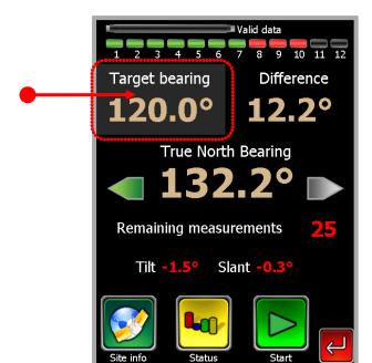
Before starting the measurement first set the **Target bearing** by pressing the area in the top left.
