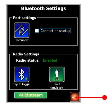
**Note:** Only one PDA can connect to a **SPAA05** tool at any time. The **SPAA05** Bluetooth is hidden automatically after connection. So if no **SPAA05** tool is found, make sure that no other PDA's are connected to the **SPAA05** tool.
