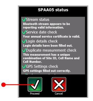
The measurement will now start. You will go back to the **Start Measuring** and the **Remaining measurements** will count down. Do not move the antenna with **SPAA05** tool until the **Measurement succeeded** message has popped up.
