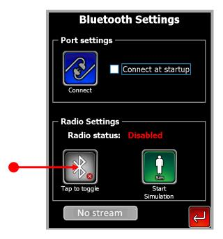
When **Radio status** is **Enabled**, press on the **Connect** button to make connection with a **SPAA05** tool.
