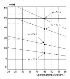
Current derating curves as a function of ambient temperature (IN = nominal current at  $45^{\circ}$ C)
