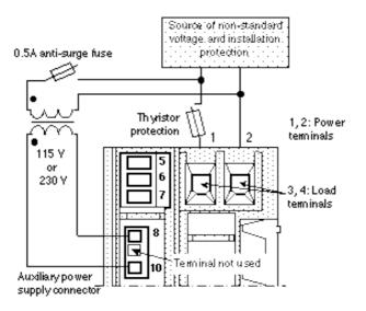
Example of auxiliary power supply wiring with non-standard mains.
