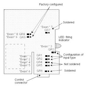
Layout of "Coffee beans" on circuit board (solder side view) GR8 and GR9 'Coffee beans' are configured in the factory GR6 and GR7 'Coffee beans' are soldered GR4 and GR5 'Coffee beans' are not soldered
