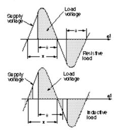
Load voltage in 'phase angle' firing mode  $(\theta)$ : thyristor firing angle)
