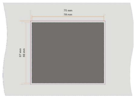
Hole dimension: 79mm\*67mm(width\*height), the dash line frame is the controller dimension. The controller is fixed by six specially customized fasteners.
