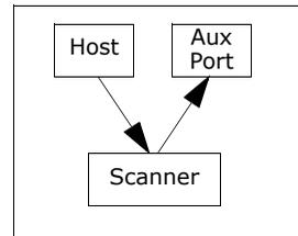
*Serial Cmd:* **<K101,aux port mode,baud rate,parity,stop bits,data bits,daisy chain ID status,daisy chain ID>**
