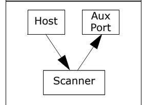
*Serial Cmd:* **<K101,aux port mode,baud rate,parity,stop bits,data bits,daisy chain ID status,daisy chain ID>**
