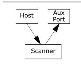
*Serial Cmd:* **<K101,aux port mode,baud rate,parity,stop bits,data bits,daisy chain ID status,daisy chain ID>**
