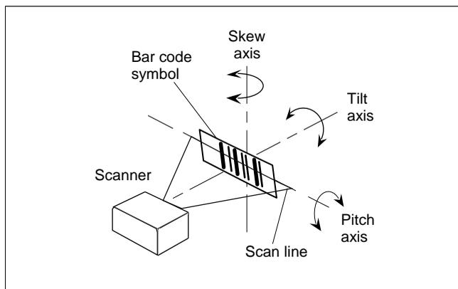
Figure 1-3 Symbol/Scanner Position
