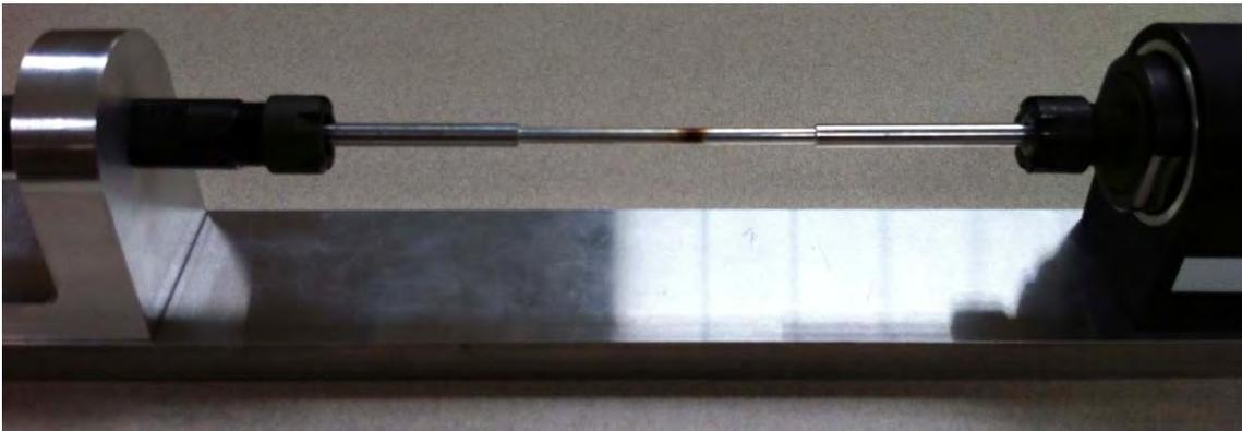
**Figure C4 – Heater tube positioning**
