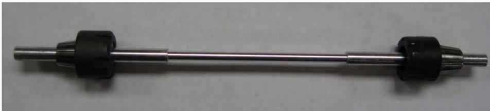
Figure C2 – Collets on heater tube
