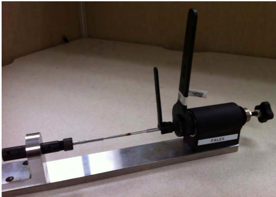
**Figure C6 – Tightening right collet**
