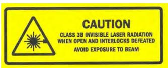
**LASER INTERLOCK CAUTION:** This label indicates exposure to laser radiation is possible when access door is open and safety interlocks are defeated.
