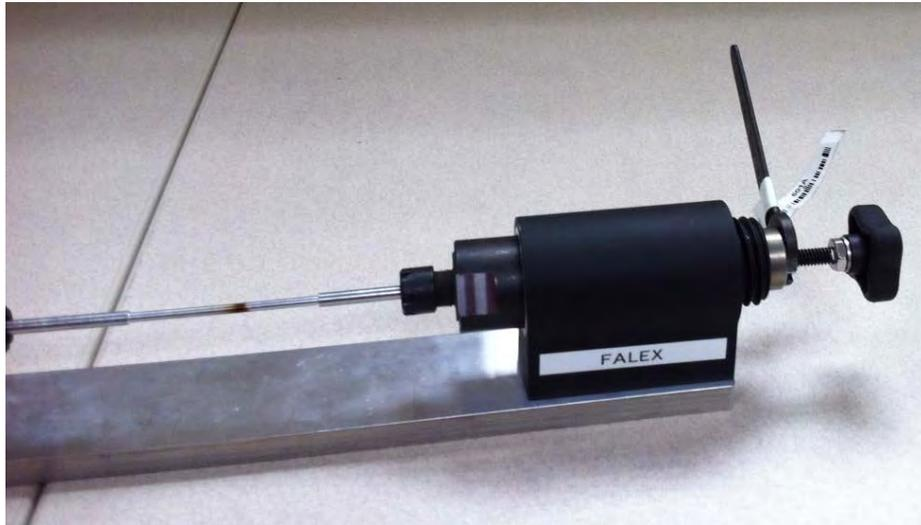
**Figure C7 – Tightening right collet**
