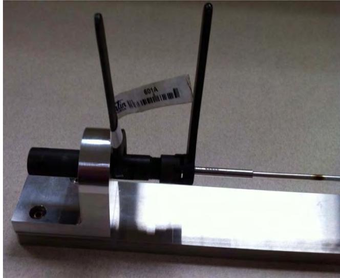
**Figure C5 – Tightening left collet**
