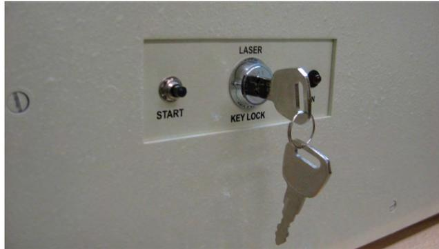
**Figure 7 – Laser Power Key Switch in 'Off' Position**
