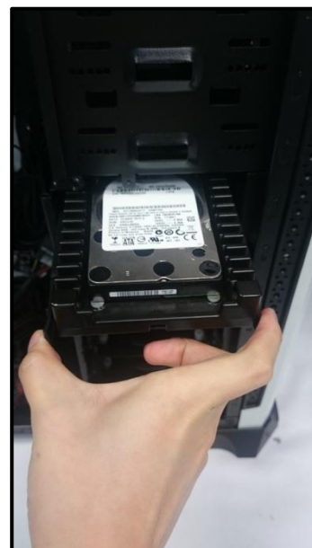
Pinch the ends of the tray and insert your drive until it clicks.
