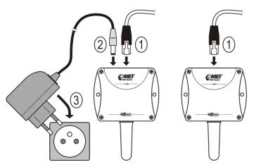
Web Sensor P8631 connection (power supply adapter, Power over Ethernet):
