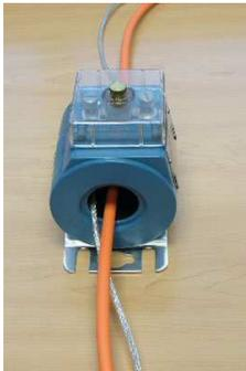
Feed the 10 or 30 ft additional wire through the ct. Connect to the second box, following current flow conventions. Can put as many loops as needed for additional current testing.
