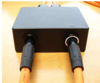
Ensure the plugs are pushed in firmly. To remove the plugs, push in, then pull out. The connector with the white circle is return.
