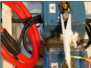
Wrap probe around all conductors
