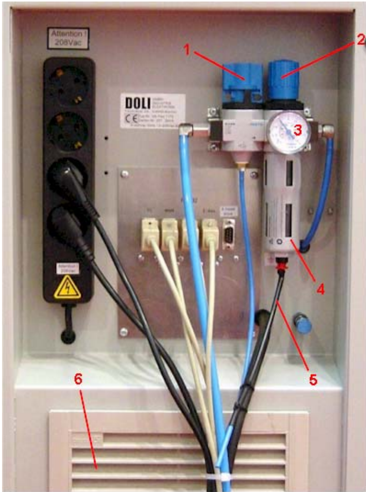
Fig. 52: Compressed-air unit and outlet box in the back of the instrument. 1=compressed-air valve, 2=compressed-air setting valve, 3=compressed-air display, 4=water separator, 5=water separator valve, 6=maintenance access for the filter mat.
