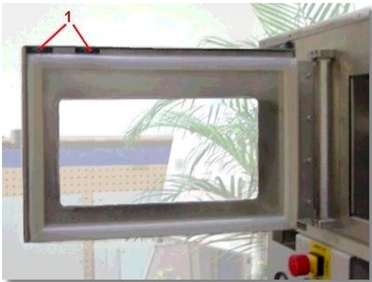
Fig. 12: Front door of the temperature chamber, open. 1=security sensors.
