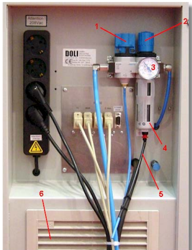
Fig. 16: Front view of the Flexometer (trimmed area, covering removed). 1=main switch, 2=emergency-stop, 3=Compressed-air display, 4=temperature chamber, 5=chamber display, 6=fan-switch
