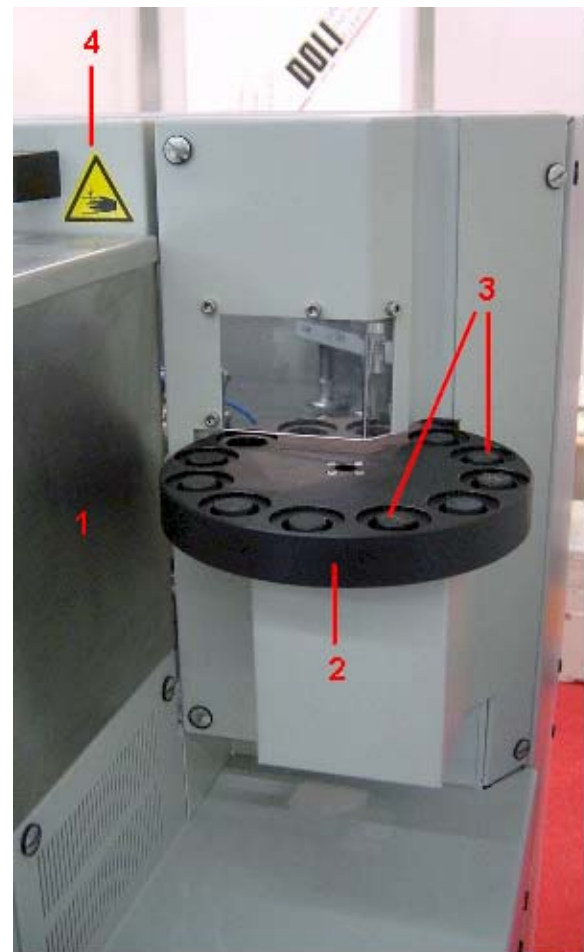
Fig. 4: Input Station of the Flexometer. 1=Temperature chamber (side wall), 2=input station (with 9 samples), 3=samples, 4=Magazine lid.
