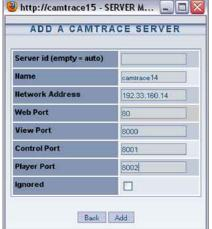
Connect to the administration web interface then click on servers. The server manager window appears with contains the list of cluster servers (two in our example). Click on 'add a CamTrace server' to declare a new server. Leave the server id empty. It will be allocated automatically. The ports specified are the default ports.
