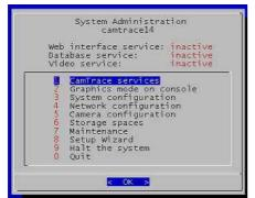
Go to the menu "Network configuration". In the submenu "Network interface configuration" enter the IP address, mask values and leave empty the maximum bandwidth state.
