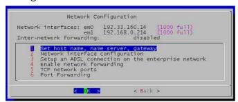
To test the configuration, go to the "Quit" menu and perform a ping on the IP address of a local network station:
