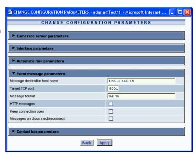
If the CamTrace Supervisor is located behind a router, you must enter the public IP address of the router on the WAN side and activate the address translation (NAT) in the router.
