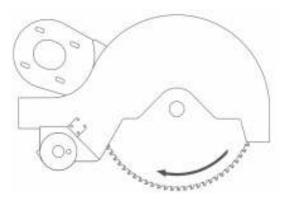
To correct the rotation direction of the saw blade, insert the electric power socket of the machine to the 3-phase slot, which has been prepared before, and follow these instructions:
