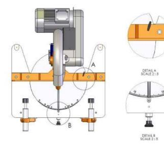
DETAIL A: Intermediate angle setting screw DETAIL B: Angle display scale The table can be fixed at any desired intermediate angle using the scew. At intermediate angles the snap pin is not in locked position. The machine table is tightened only temporarily.
