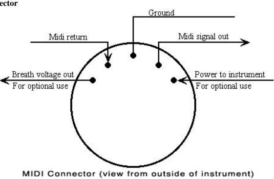
The power applied to the power input pin can be anywhere between +7.5 and +12 vdc and must supply at least 15ma.
