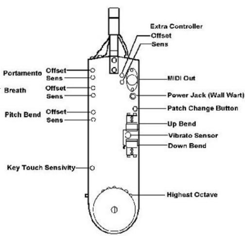
As you can see, the parameter trimmers are in pairs and consist of a SENS (sensitivity) trimmer and an OFFSET trimmer. Of each pair, the OFFSET trimmer is always closest to the mouthpiece end. It is good to get this planted firmly in your mind so that you stay away from accidentally changing a Sensitivity trimmer. If you have a good understanding of the concept of offset and sensitivity, then you should not have much difficulty in making adjustments to any of the trimmers.
