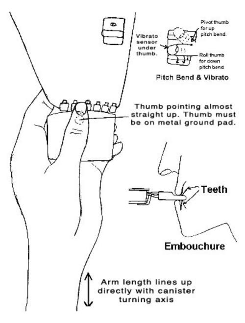
The Electronic Woodwind Instruments have two more rollers since the thumb needs something to rest on in the bottom octave. The pitch range is the same as the EVI. The AKAI EVI's have an extra roller on the bottom but it is a dummy and has the same pitch range.
