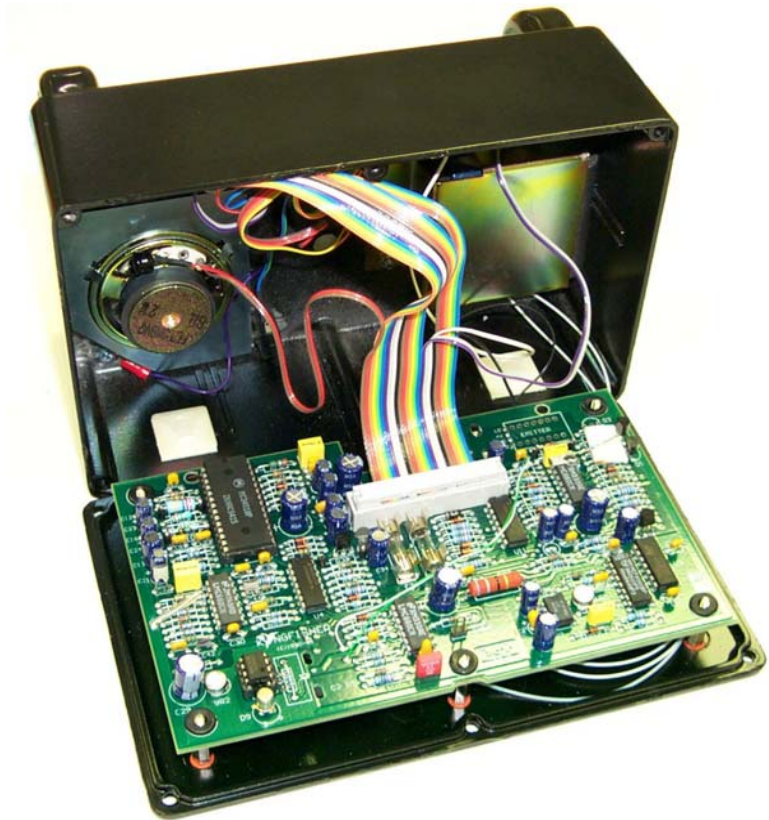
Figure 3 KI 025DD Optical Talk Set, Internal View
