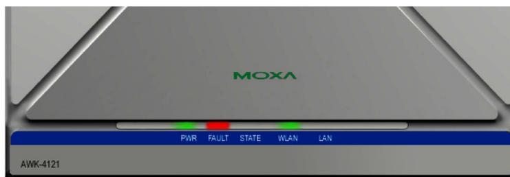
The following table is a summary for the wireless settings and LED displays. You can check the status of the AWK-4121 by reading these LEDs. More information about "Basic Wireless Settings" is presented in Chapter 3.
