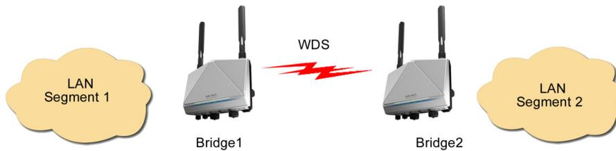
It is a good idea to plan your wireless network by drawing a diagram so that you know how each AWK-4121 is connected to other peer APs or wireless bridges by WDS, and how bridges are connected to other peer bridges by WDS. See the following figure for an example of a network-planning diagram.
