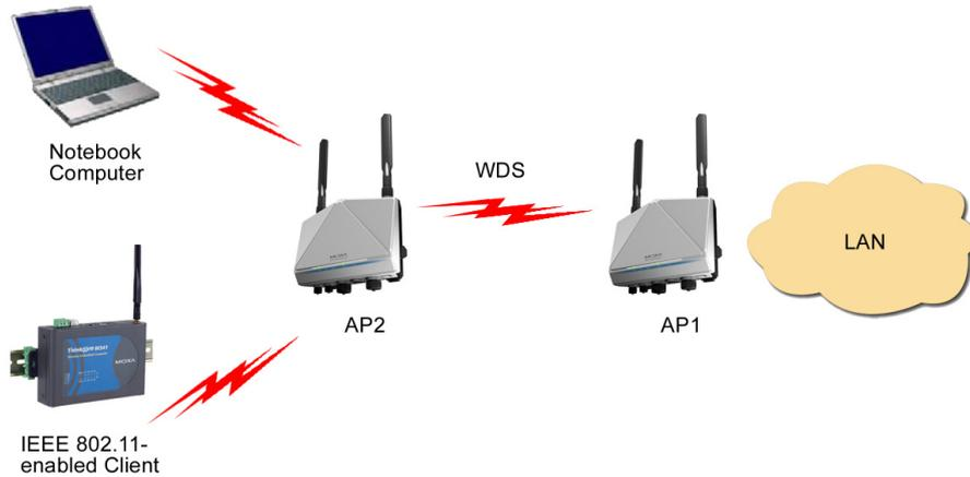
By using WDS, two or more LAN segments can be connected wirelessly. As illustrated in the above figure, a pair of wireless LAN-to-LAN bridges is used to connect two LAN segments. Since the AP is WDS-enabled, it can be used as a wireless bridge.
