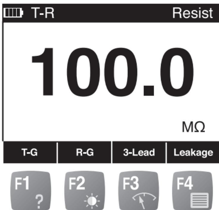
The initial LCD screen displays single pair resistance for tip-to-ring. The function keys have the following choices:
