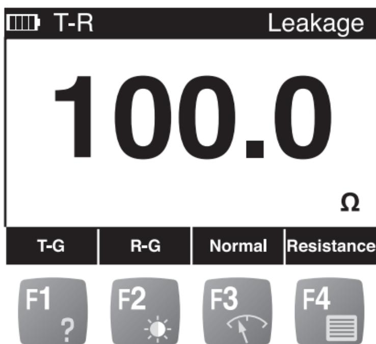
The leakage measurement for a single pair appears in the LCD. The measurement updates continuously. The Leakage test also has the option to reverse the polarity of the 135 VDC by pressing **F3 REV**.
